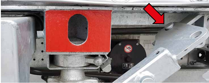
Photo 84c Properly attached brace
